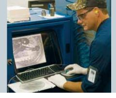
Christopher Hyde operates a turning lathe to machine the outside diameter of a dollar coin reverse die. He can watch the machining process on-screen.
