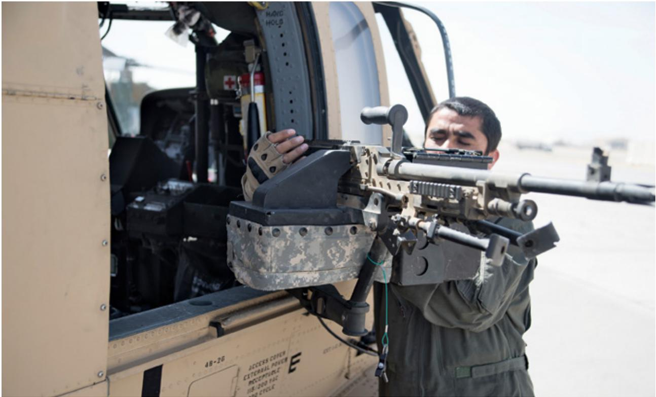
**An Afghan Air Force UH-60 crewmember attaches his M240 machine gun during a preflight inspection.**
