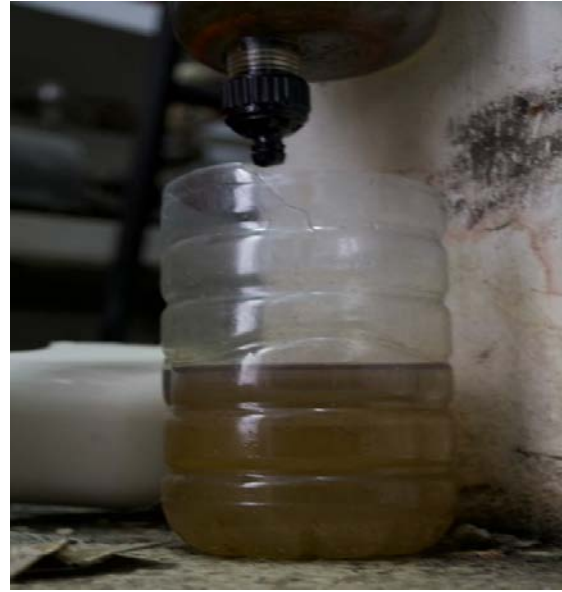
Figure 2: Sediment in diesel fuel extracted from a generator at Embassy Ankara, Turkey. (OIG photo, Oct. 2018)
