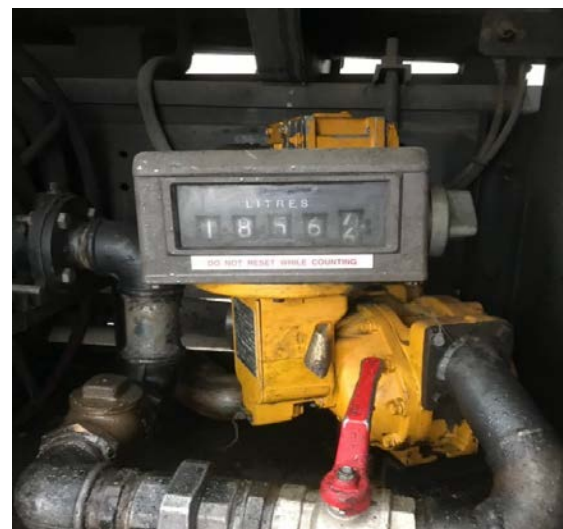
Figure 3: Flow meter on contractor's delivery truck at Embassy Beirut, Lebanon. (OIG photo, Dec. 2018)
