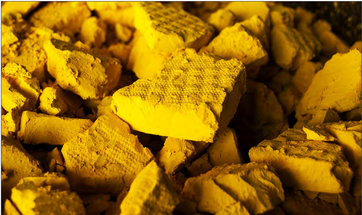
A photo of yellow cake uranium, a solid form of uranium oxide produced from uranium ore. Yellow cake must be processed further before it is made into nuclear fuel. Courtesy of Energy Fuels Inc.
