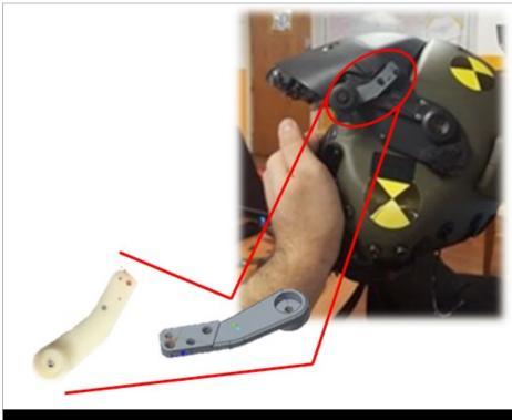
Figure 7. AM-Produced H-1 Helmet Visor Clip Source: The Marine Corps.
