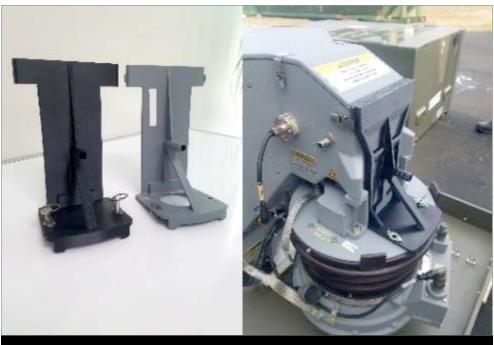
Figure 4. Traditionally Manufactured and AM-Produced MH-60R Airborne Low Frequency Sonar Covers
