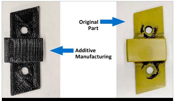
Figure 8. Traditionally and AM Produced Bump Stops for F-35B Landing Gear Door Source: The Marine Corps.
