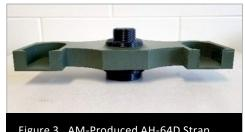
Figure 3. AM-Produced AH-64D Strap Pack Support Source: The Army.
