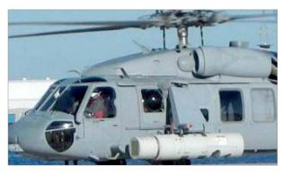
Airborne Laser Mine Detection System
