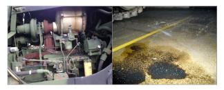
Photos of Full-Tracked Tractor with Engine Corrosion (left) and Armored Bridge Vehicle Class III Leak (right)
