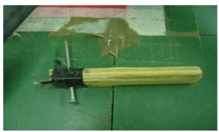
Figure 8: "Screw tool" used to strip Kevlar
