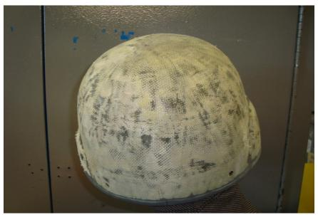
Figure 9: Damaged ACH after paint removal.
