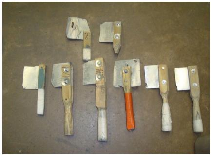
Figure 7: Hatchets used to remove paint.
