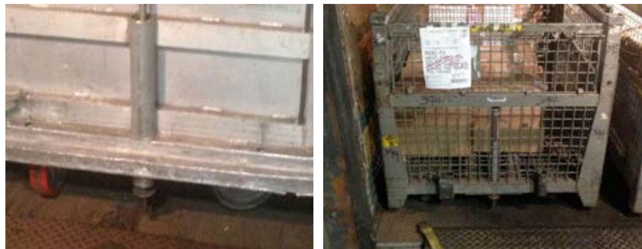
Figure 9. Large OTR Container and Wire Cage Not Secured in Trailers at the Chicago NDC
