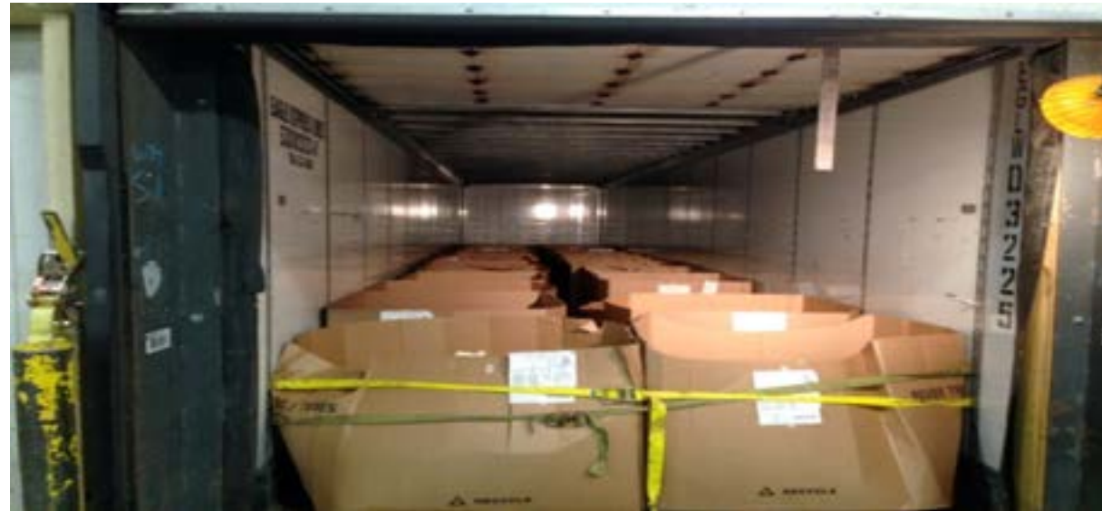
Figure 8. Inadequate Number of Load Restraining Straps
