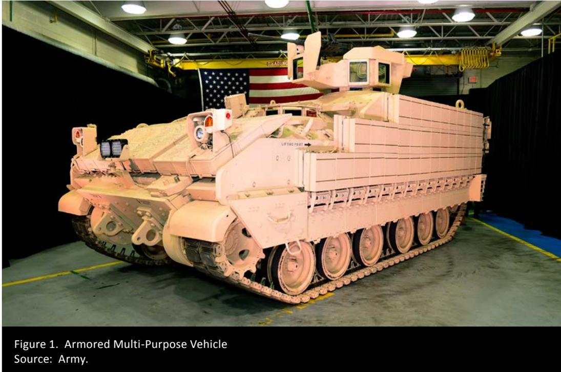
Figure 1. Armored Multi-Purpose Vehicle
